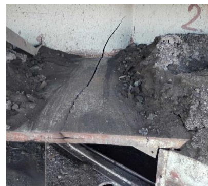
Figure 1. a) Slewing platform horizontal plates, workload, stress distribution (Note: 13.2 kN/cm 2 equals to 132 MPa), b) A crack on a lower horizontal plate of a slewing platform
