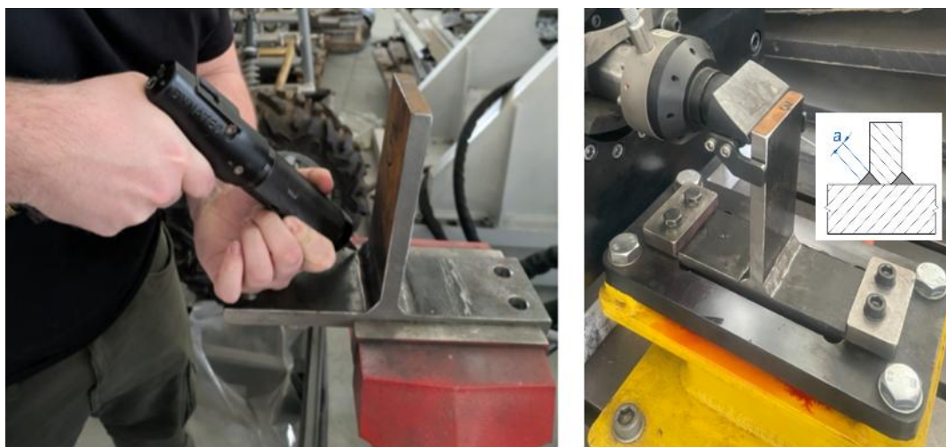
Figure 1. Application of HFMI technology and a test specimen in the test stand
