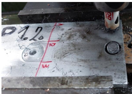
Figure 1. Cutting samples for measuring electrical conductivity
