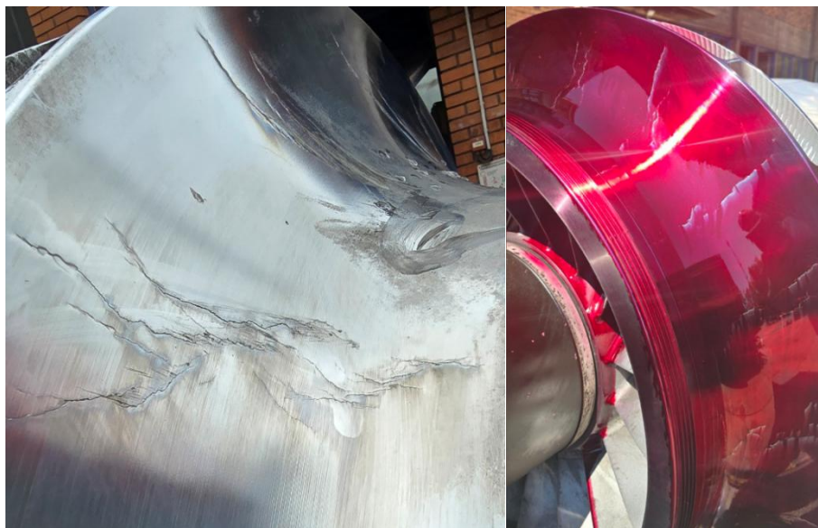
Figure 1. Cracks in 2nd stage impeller of an air compressor
